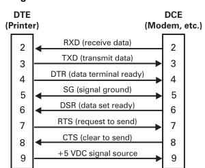
Figure 46 • RS-232 Cable Connections
